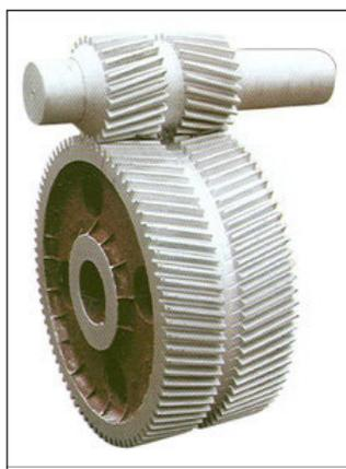
Figure 8-5: Double helical gear sets use two pairs of opposed gear teeth to eliminate thrust load
